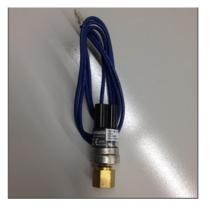
**Low Pressure Switch:** The low pressure switch is an automatic reset that senses compressor suction line pressure. In early production models, it opens at 40 PSIG and control closes at 80 PSIG. In the latest productions models, it opens at 10 PSIG and control closes at 25 PSIG.
