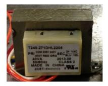
**<u>Control Transformer:</u>** The control transformer is rated at 24 vac, 40 va (1.6 amps @ 24vac).
