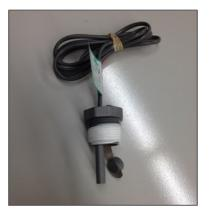
**Flow Switch:** The flow switch senses liquid solution flow. The paddle of the switch is inserted through a fitting into the pump discharge line. Liquid solution flow deflects the paddle and closing the switch. The flow switch is position sensitive. The arrow ↑ on the switch must point in the direction of liquid solution flow. Maximum flow is not to exceed 28.8GPM
