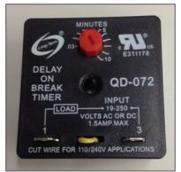
**System Delay Timer:** The refrigerant timer is a 24 vac, 5-minute delay on break timer. The normally closed contacts of the timer energize the compressor contactor through the chilled liquid solution control. When the chilled liquid solution control contact opens, the timer delays by opening its contact for 5 minutes before resetting to the closed position.
