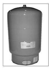
**Supply Storage Tank:** A supply storage tank must be used in a system with less than 50 gallons or 5 gallons per ton - whichever is greater - of liquid solution. The tank prevents rapid cycling of the compressors and acts as a reservoir for chilled liquid solution.
