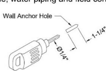
Drill diameter 1/4" depth 1-1/4" holes
